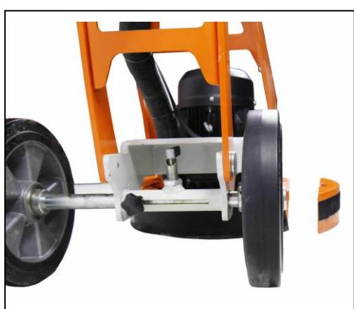
Subsequently turn the locking bout on the chassis with the handle into the upper position and then loosen the star grip screw. You can now move the machine to the right or the left using the handle so that the chassis shifts aside and you can grind flush wall. Then secure the chassis by engaging the locking bout in the desired position.
