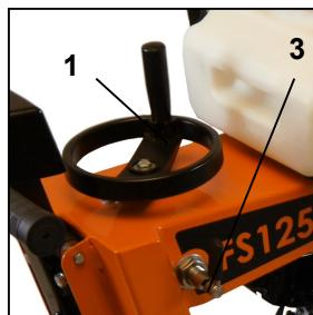
Connect the water supply and slowly lower the machine with the hand wheel (1) till the blade has ground contact. Putting down the machine to the desired cutting depth which is displaying on the cutting depth indicator (2).
