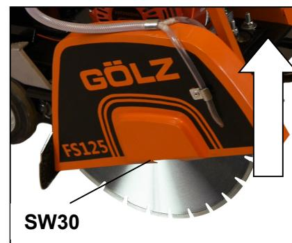
Remove the cutting disc guard and unscrew the outer clamping flange SW 30, left-hand thread.
