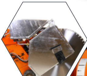
Divisible blade guard - can be raised for intersections
