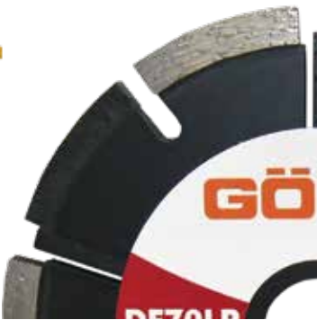
DF70LR Diamond raking blade • Offset segments and TCT protection segments • Undercut protection segments • Brickwork, joints
